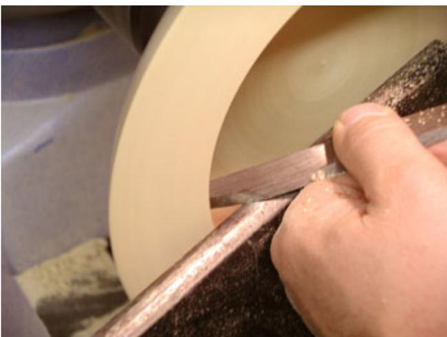
11. This shows how far the rim is undercut. Notice that the tool is pointing down and that it is flat on the tool rest - very important!
