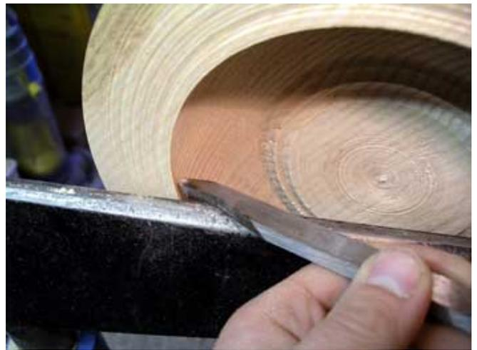
10. This is the tool to undercut the rim. This one is home made out of an old scraper. These are commercially available under the name of "Hook" tools. This is sharpened like a scraper using a burr formed by grinding to act as the cutting edge.
