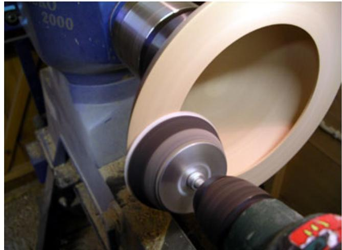
12. Here I am power sanding the rim with a 3" sanding pad and a 120 grit abrasive disc. The rest of the inside is sanded to 600 grit.
