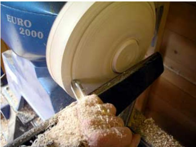
3. Here the back of the bowl is starting to be shaped. A 60mm spigot has been cut using a parting tool in preparation for the chuck jaws.
