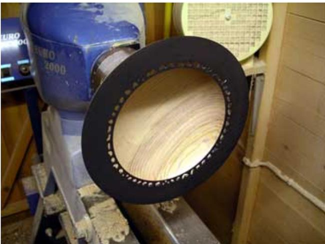
17. The dye has now been completely applied to the top surface.
