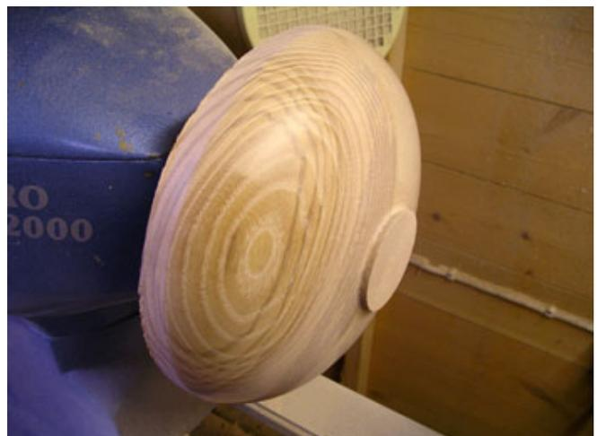
6. The finished back of the bowl after sanding. I start with 150 grit cloth back abrasive and work up to 600 grit. Make sure that you don't miss out any grades!
