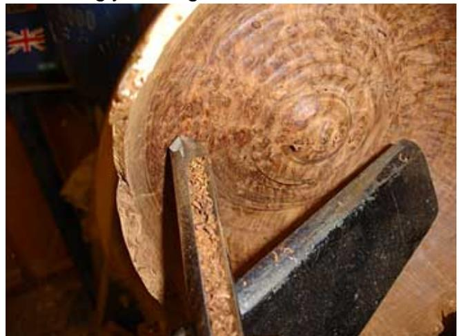
22. Back to reducing the wall thickness using a push cut. The wall thickness is only about 5mm thick so be very careful at this point because it is very easy to go thinner at this point as the bowl turns in near the bottom.
