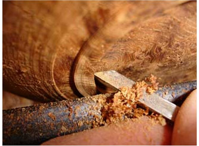
8. Now I use a "9 in 1" tool to create the dovetail in the bottom. Always make sure that this tool is sharp otherwise it will tear the grain and it is difficult to sand this area properly.
