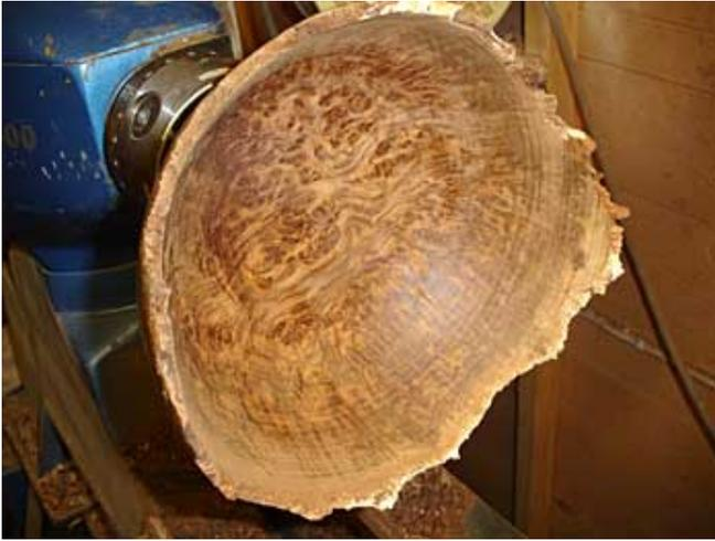
23. The finished inside of the bowl which is now ready for sanding. The ridges that are visible are caused by the length of the grind on the chisel. Normally they can be removed by using the 1/4" bowl gouge with a short bevel. As they were not deep I decided to sand them out
