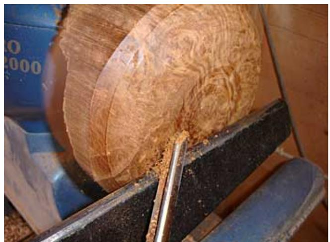
6. The bottom face is now cleaned up using a pull cut with a 1/2" long grind bowl gouge. At this stage I am only roughly cutting it to size, I am not too bothered about the finish.
