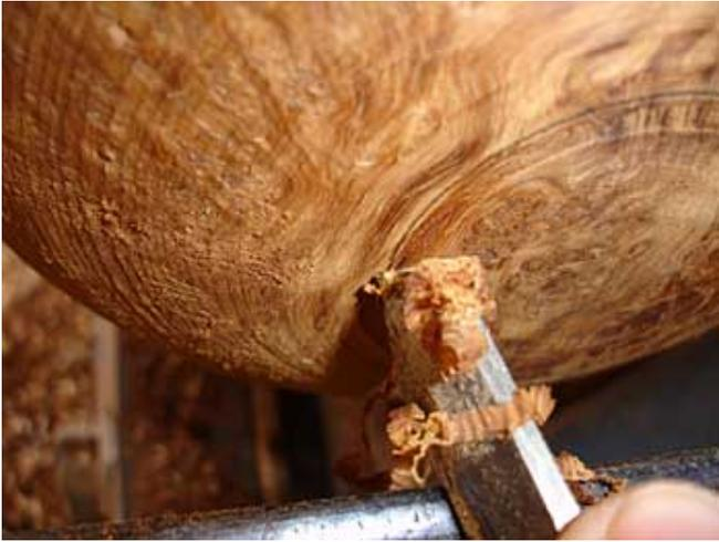
7. When I turn the inside of the bowl I will be using chuck jaws in an expansion fitting. Here I am using a parting tool to make the first cuts.
