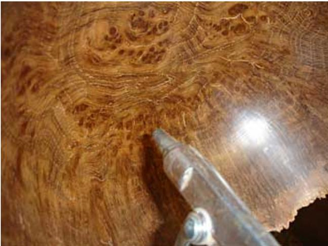
25. After sanding up to 600 grit, use a compressed air gun to remove all the dust from the crevices and on the natural edge.
