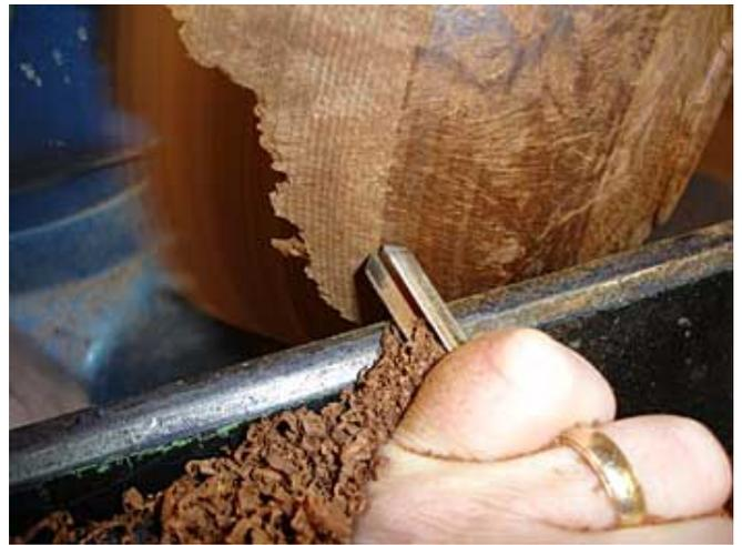
10. A 1/4" standard grind bowl gouge is freshly sharpened and 2 very fine cuts are made. You can see the difference already.
