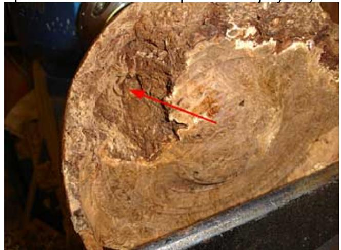
20. After removing a large piece of bark, it revealed a large hole (as shown by the red arrow). I decided to make the wall thinner than anticipated and hopefully it should turn out the ugly looking hole.
