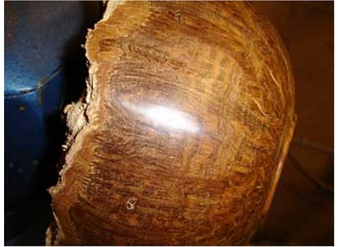
14. Sand up to 600 grit without missing any grades. I have not applied any oil or sanding sealer at this stage, the shine is from the newly sanded wood.
