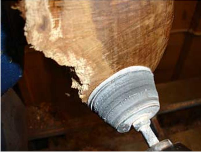
13. Start sanding using a Velcro backed sanding system. This is the safest way to sand the natural edges. The sanding pad must be kept as close to 90 degrees as possible to the work but without the work catching the pad. Also do not use too much pressure, all this advice is for safety and to prevent any edges being rounded over.
