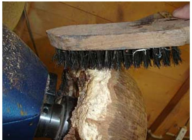
12. Here I have had to use a wire brush to remove the dead bark and sap wood which had turned white. Do this with the lathe stationary and before sanding otherwise the wire brush will scratch your newly sanded finish.
