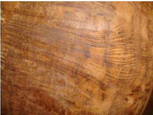
11. This after the fine cuts have been taken. This photo is the same area as the photo above. As you can see this type of cut virtually eliminates all the torn grain.
