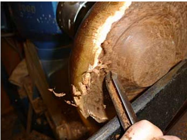
21. Try to keep as much material in the centre as possible, this will help stabilise the thin walls. Reduce the thickness in stages from the edge to the centre. Here I am cutting back the centre with a right to left cut in preparation for the next stage of cutting.
