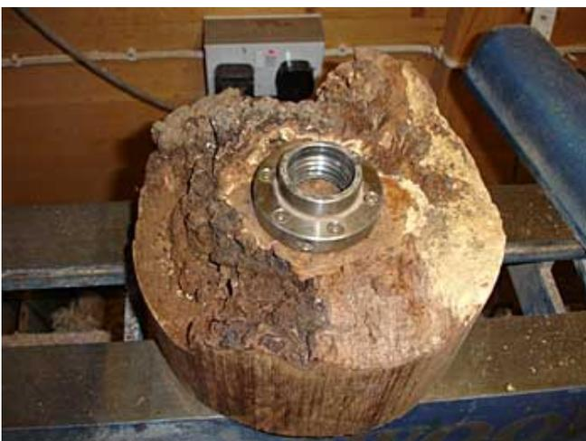
5. The screw chuck is now securely in place. All the screw holes were used because this type of wood will always be out of balance on the lathe and it needs all the support possible.
