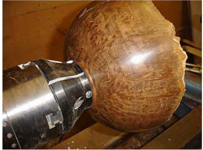
18. Always check to make sure that it does not split the wood on the mounting point because the initial cuts on the uneven top surface will make the point fail with spectacular results and possible injury to you.
