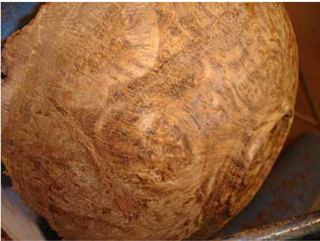
9. The outside of the bowl has now been turned to the finished shape but the grain is quite badly torn due to soft patches in the wood and fairly heavy cuts.
