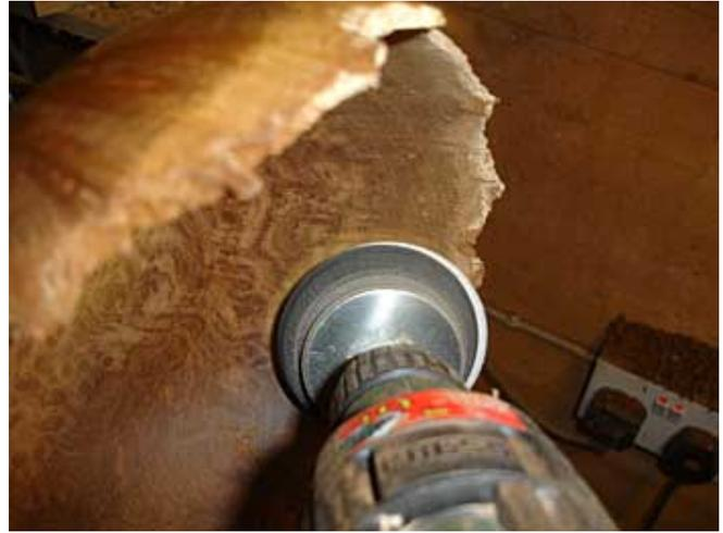
24. Sand using the Velcro backed abrasive system using the same technique as used for the outside of the bowl.
