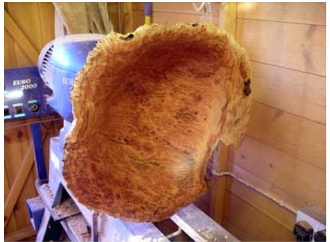
15. The finished inside after applying the sanding sealer. Now the whole bowl is polished, buffed and then waxed with pure carnauba wax. This wax is very hard.
