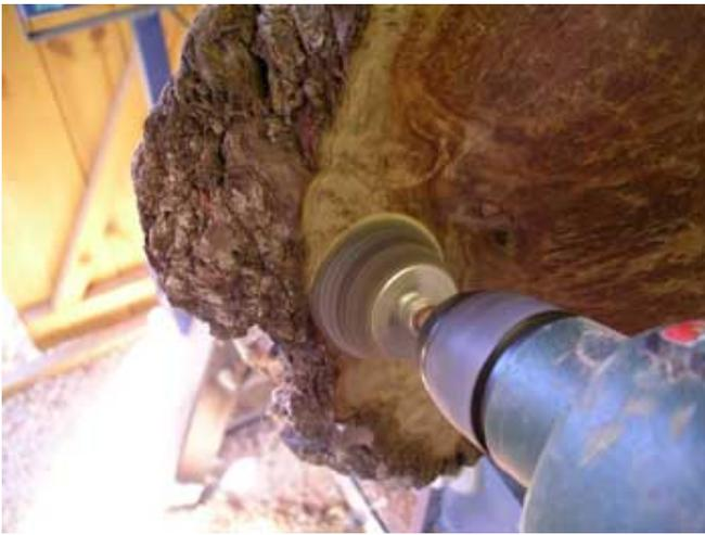
6. Power sand the overhanging natural edge with a 2" Velcro pad with the bowl stationary. You do not want the moving bowl to grab the sanding pad and draw it into the moving bowl.
