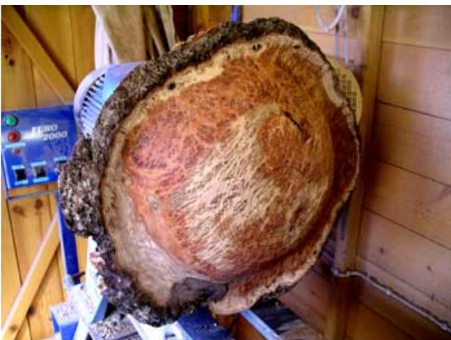
4. The back has now been completed using the 1/2" bowl gouge. You can just make out the marking of the foot in pencil. The foot is cut using a parting tool and 1/4" spindle gouge.
