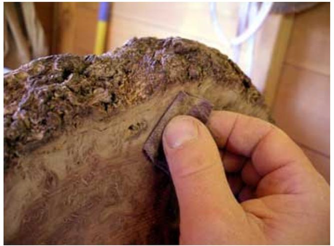
7. After power sanding, hand sand the natural edge. The rest of the back of the bowl can be sanded with the bowl moving.
