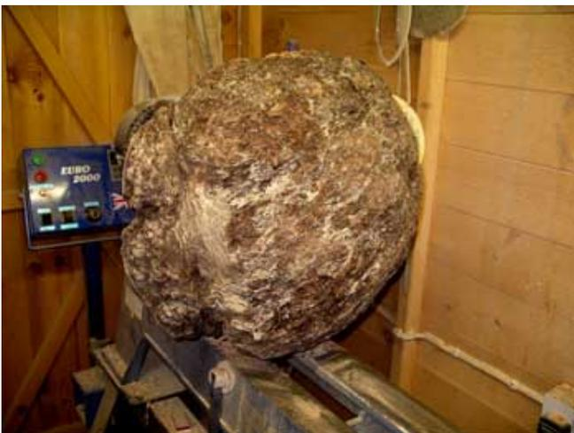
2. The reverse side showing the bark which is still intact. If the bark is loose I usually remove as much of the bark as possible before turning otherwise it tends to fly off! In this case the bark was very tight.
