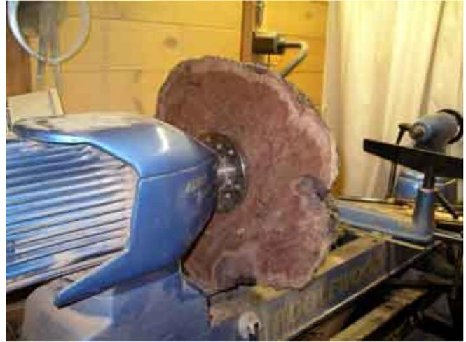
1. The piece of timber weighed 19.2Kgs and was 20" across at it widest point. I used a 6" face plate to mount the piece on the lathe.
