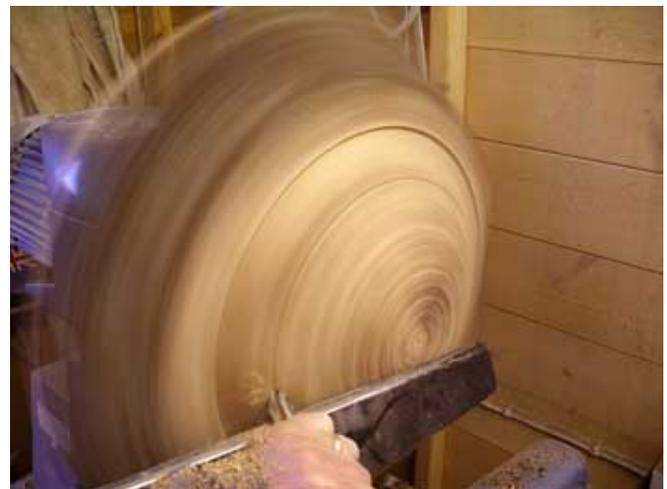
3. With speed of the lathe at about 350rpm the back is starting to be turned. **WARNING!** Keep all loose clothing out of the way of the natural edge; it could quite easily snatch any loose clothing, hair etc!
