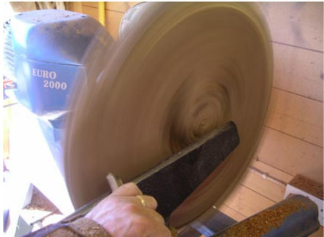
11. Turning the inside at around 400rpm using the 1/2" bowl gouge. Watch your fingers!
