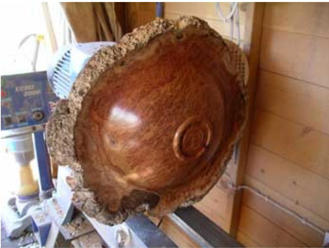
8. The finished back of the bowl. This photo was taken after sanding and 2 coats of sanding sealer applied.
