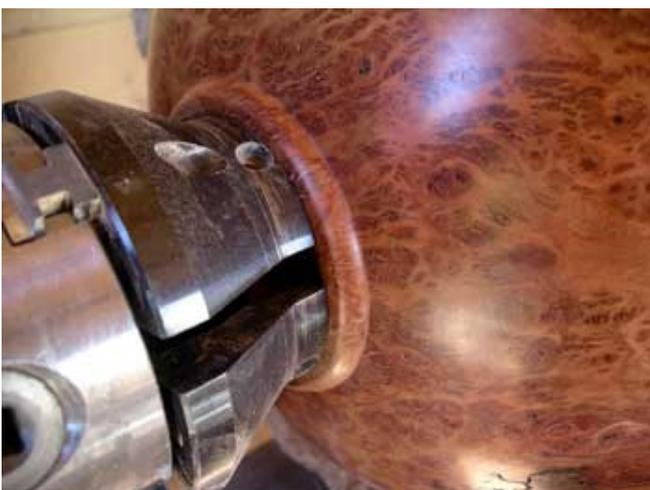
10. Close up of the way that the jaws are gripping the inside of the foot. A good fit is essential especially on a bowl this size.
