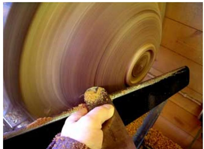
5. The problem with the bowl gouge on very hard timbers like this is that it tends to tear the grain. The solution is to use a big scraper to take fine cuts and smooth the outside and so reduce sanding.
