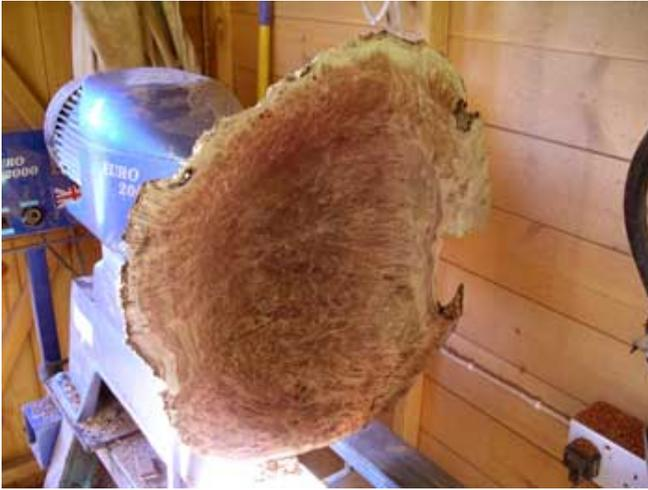
12. The inside is now finished. To achieve a better finish than the bowl gouge, use a scraper to remove the torn grain as before. Sand again to 600 grit.
